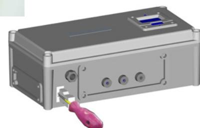
**A screwdriver must be used to disconnect the cabinet connector if the compressor is being disassembled!**
